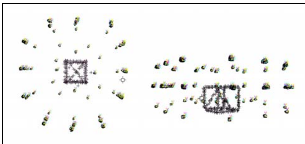
Figure 4. Bundle design containing 120 images, top and front view.
