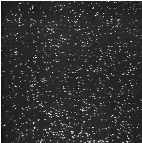
Figure 1. PTV image with ~ 1000 particles
