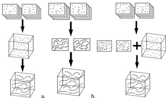
Figure 3. 3-D PTV with 3-D priority (a.), tracking priority (b.) and integrated spatio-temporal matching (c.) (Willneff, 2003)
