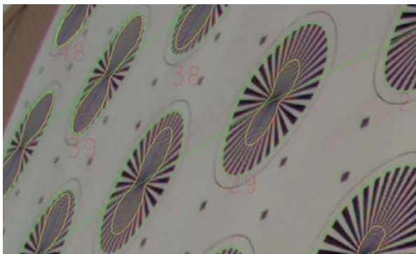
Figure 2. Fragment of photo of Siemens star test took with digital camera Kodak DCS 14nPro (10.5 mm) with broadening rings
