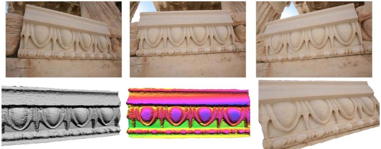
Figure 7. Results of the multi-image dense matching reconstruction from the Canon data (0.3 mm GSD, 25-30 deg convergence angle) of a detailed area of new marble (ca. 560 x 220 mm) imaged in three images. 3D results presented in shaded, colour-coded and textured mode.
