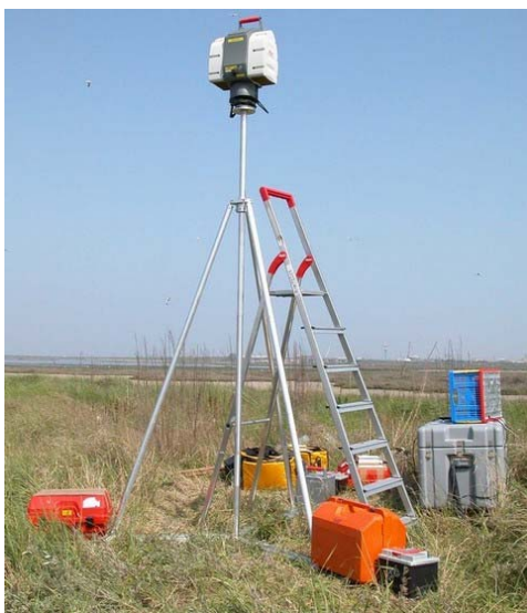
Figure 3. The tripod used to rise up the laser scanner.
