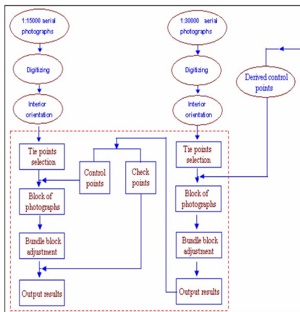
Figure 2.3 The work flow of multi-scale bundle block adjustment
