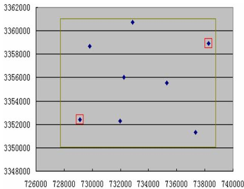
Figure 1.2 Control point distribution. Points in red frame are full control points while others are height control points. The outline indicates the entire area of KVR orthophoto.
