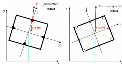
Figure 2.4 The relationship between pixel coordinate system and image coordinate system
