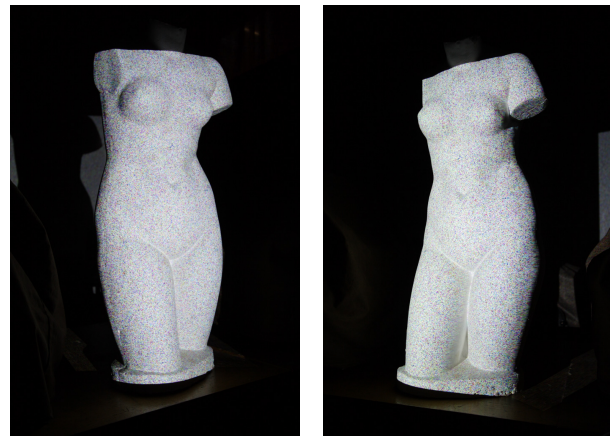
Figure1. Image correlation method for creating 3D model, using projected raster on sculpture
