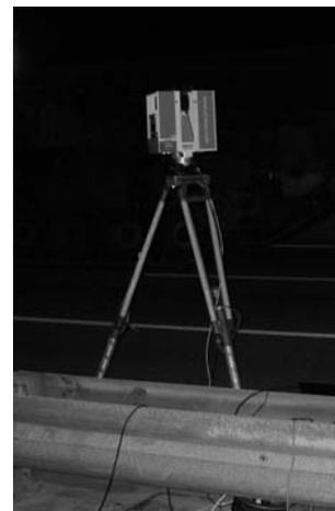
Figure 3. Terrestrial laser scanner Imager 5006 by Zoller+Froehlich (<http://www.zf-laser.com>).
