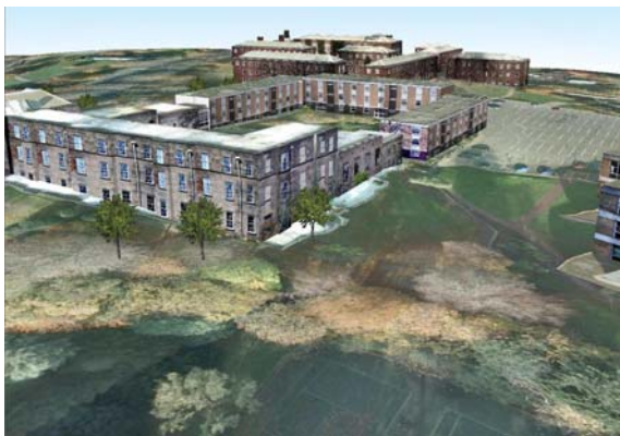
Figure 5. Student attempt to create a photorealistic 3D scene of part of the University Park Campus, using textured models, trees and ortho-images draped on DTM's.
