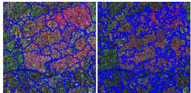
Figure 1. Comparison of segmentation results. Left: segmentation result using images derived from 8-bit transformation; Right: segmentation result using original SAR images
