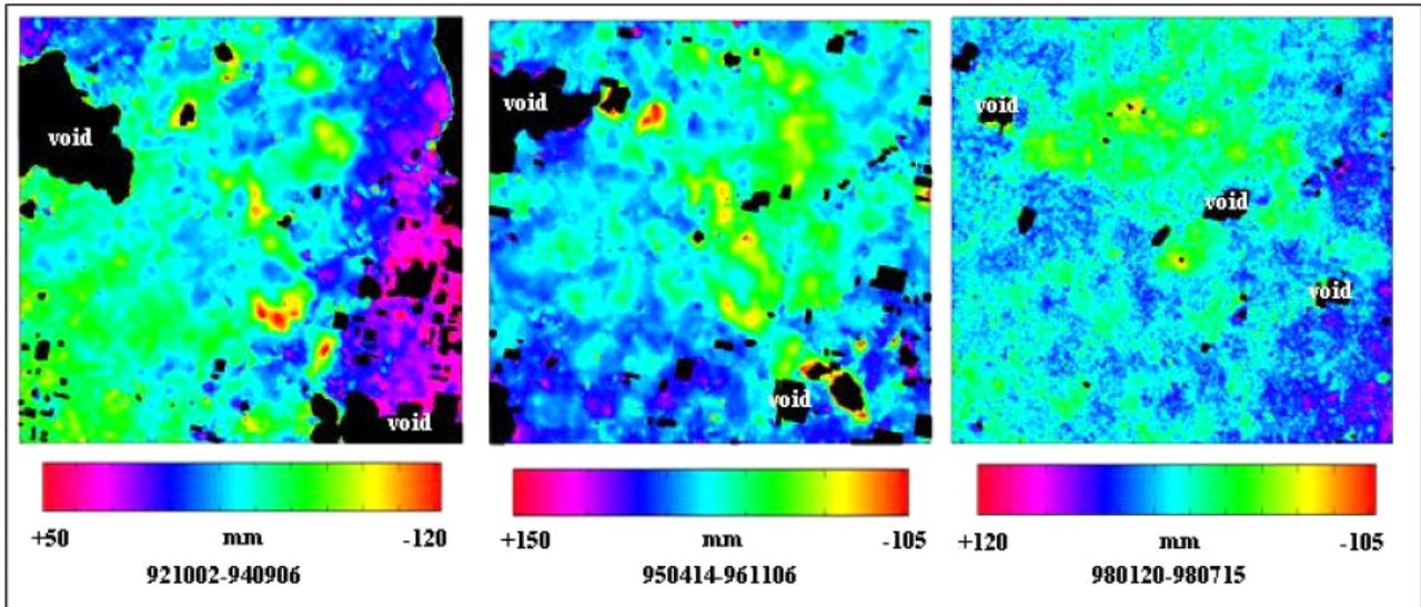
Figure 5. Deformation maps obtained from the 1<sup>st</sup>, 3<sup>rd</sup> and 5<sup>th</sup> DInSAR pairs of the series (see Table 3).
