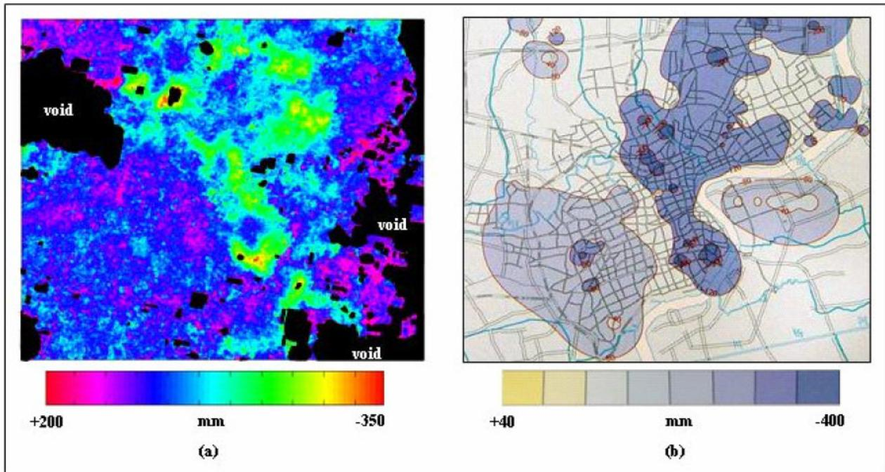
Figure 6. Accumulative land subsidence map of Shanghai: (a) obtained from cumulative sum of 5 deformation maps for the period October 1992 to July 1998; (b) obtained from land surveys for the period 1990 to 1998 (Source: Zhang et al., 2002).
