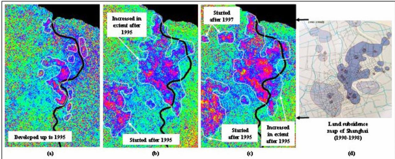
Figure 4. Developmental stages of land subsidence in Shanghai from 1992-1998 mapped by JERS-1 SAR data. (a) Stage 1: accumulative subsidence up to April 1995; (b) Stage 2: accumulative subsidence up to October 1997; (c) Stage 3: accumulative subsidence map up to August 1998; and (d) accumulative subsidence map from 1990-1998 obtained from other survey methods (Source: Zhang et al., 2002).
