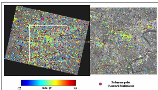
Figure 7. Deformation map obtained from PS processing using C-band ERS-1/2 SAR data over Shanghai for the period 1992 to 2001.
