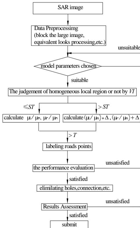
Figure 4: the flowchart of roads extraction from SAR imagery
