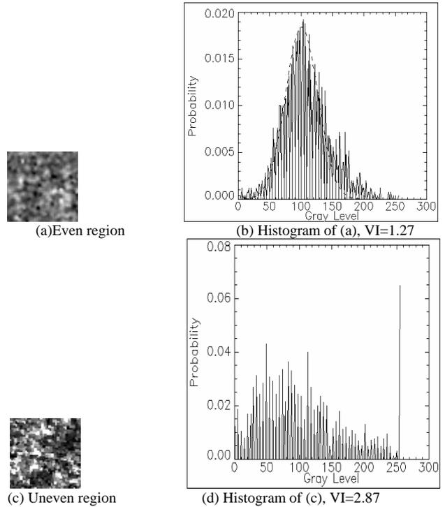
Figure 2: The typical “even” and “uneven” local region in the image, the size of local region is 50×50
