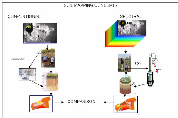
Figure 1: The concept of the optically based approach to map soil against the traditional way (Acknowledgement is given to Dr. J. Dematte for part of the illustration)
