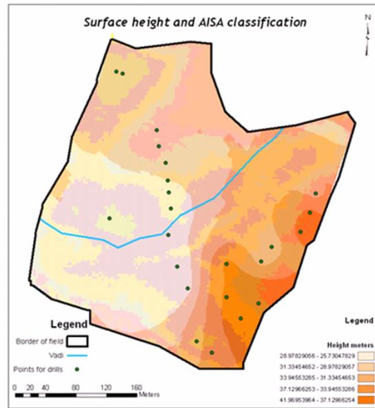
Figure 2: The ISO-Data classification of the area using the IS reflectance image overlain on the topography image of the area. Also given are the drilling point positions
