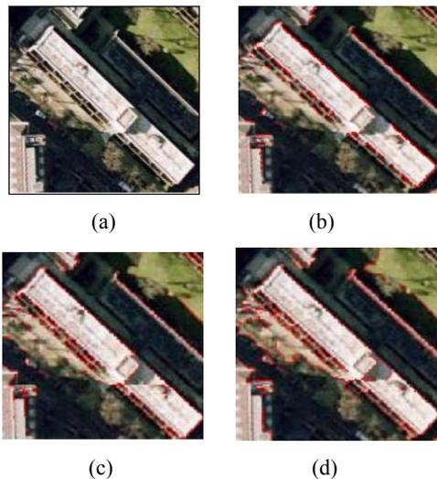
Figure.1 Several edge detection algorithm comparison (a) Removal noise Image (b) Robert operator processing image (c) Sobel operator processing image (d) Canny operator processing image
