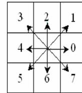
Figure.3 Eight direction coding scheme
