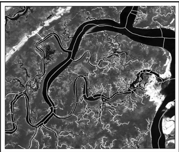
**Figure 3.** Overlaying of the NHD stream lines (in white) with the near infrared band (streams in black) of the ADAR image. While most of the large creeks are present, some other large ones and many small ones are absent. The image dimension is approximately 2953 m by 2491 m.
