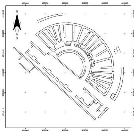
Figure 7. Photogrammetric test - Example of stereo-plotted map
