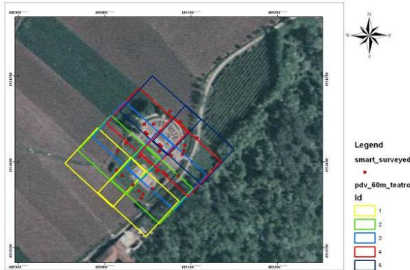
Figure 6. Photogrammetric test - Example of flight plan
