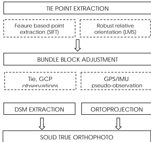
Figure 9 – Automated image processing work-flow
