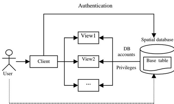
Figure 3. View-based access control mechanism for spatial database
