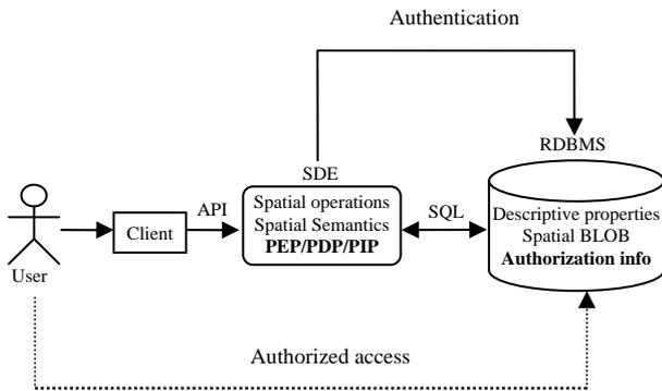
Figure 2. SDE-based access control mechanism for spatial database
