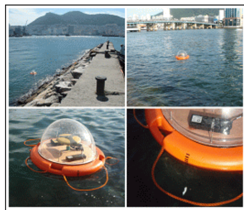
Fig. 5. Field test using GPS buoy
