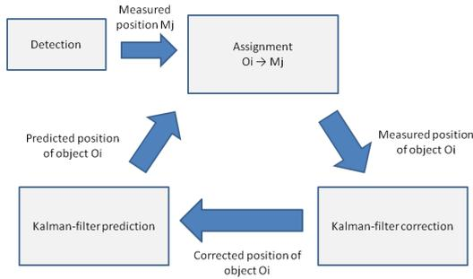
Figure 6: The steps of object assignment with Kalman-filtering
