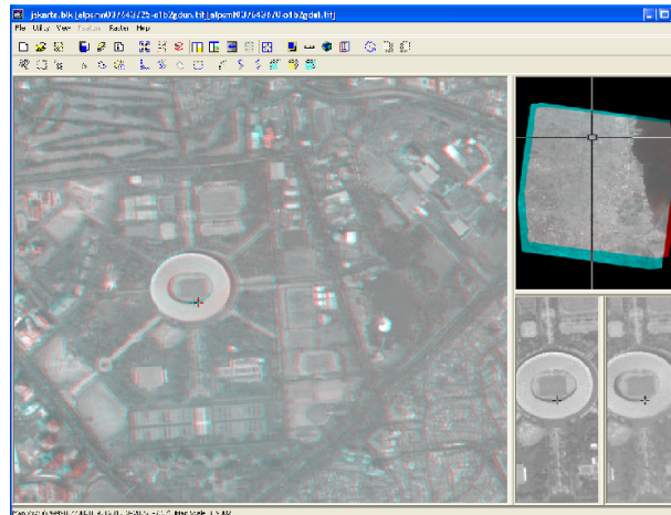
Figure 4. Anaglyph stereo display of ALOS-PRISM for Senayan area using Leica Photogrammetry Software (LPS) - Erdas Imagine
