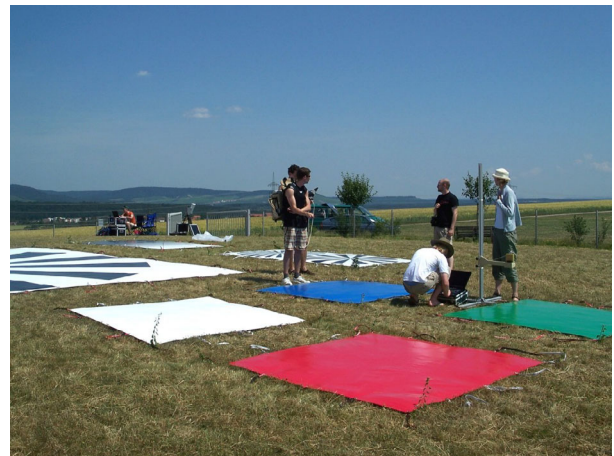
Figure 1: Ground teams performing reference measurements in radiometric test field
