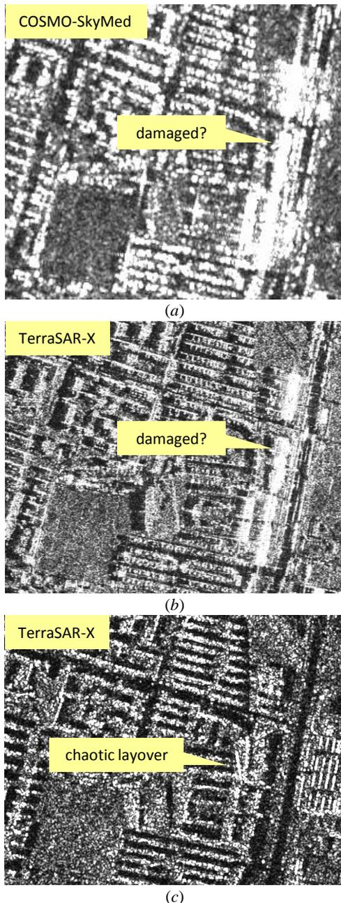
Figure 6. Descending COSMO-SkyMed image (a), descending TerraSAR-X image (b), and ascending TerraSAR-X image (c) of Dujiangyan city.
