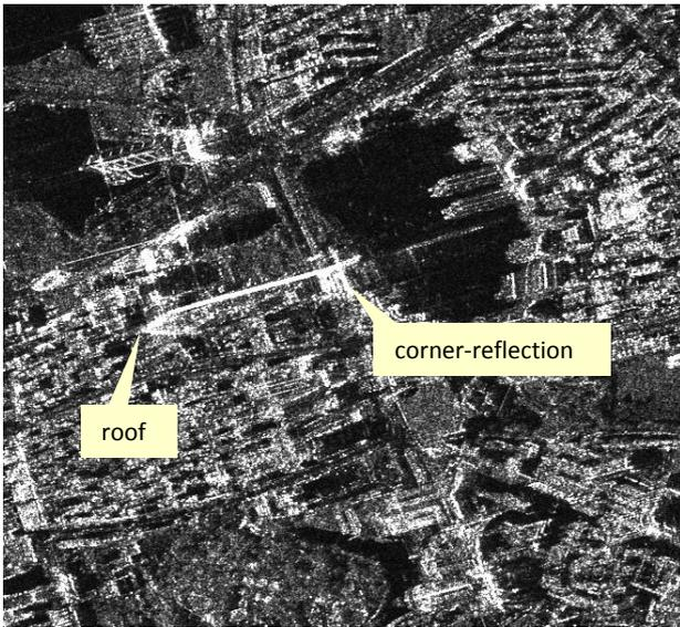
**Figure 1. TerraSAR-X spotlight image from October 31, 2008, acquired in VV polarization from an ascending orbit.**
