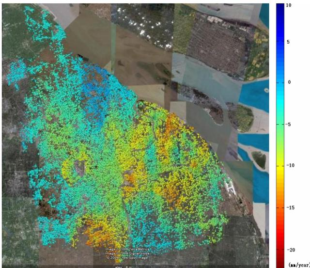
Figure 10. Subsidence measured over Shanghai using PS-InSAR.
