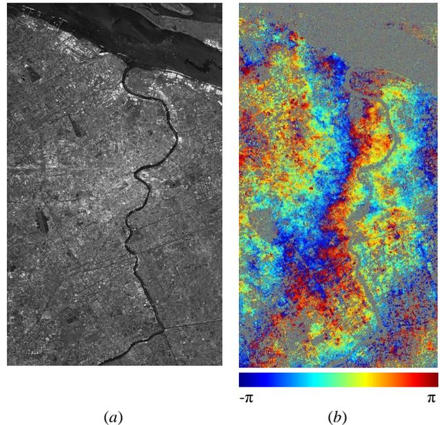
Figure 7. TerraSAR-X InSAR results over Shanghai. Amplitude image (a); Interferometric phase (b).
