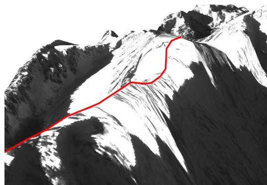
Figure 14: Example of an 'incorrectly' rectified image (the lit parts go 'over' the ridge)
