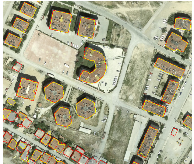
Figure 4. A small part of the ortho-image. The red polygons show the available reference data, the yellow polygons shows the results of the proposed methodology.
