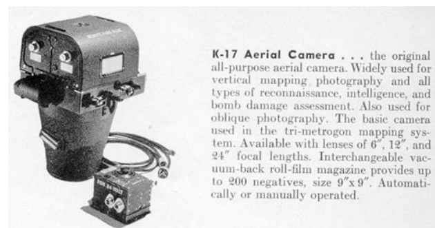
Figure 2. The Fairchild K-17 aerial camera, here with 12" focal length (Verney, 2009)
