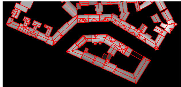
Figure 10: DEM of the “Schneiderberg” area overlaid with the corresponding vector model with height values from 0 to 23.8 meters (rescaled for visualization)
