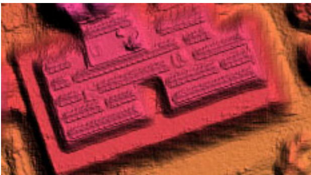
Figure 11: Example: UC-X, 8cm GSD DSM of an industrial building with solar panels on the roof.
