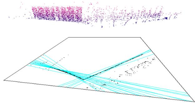
Figure 8: Two difficult facades for the classical Hough Transform: i) a curved facade, and ii) a facade with a low density of 3D points. The detected lines correspond to the local maxima of the Hough space accumulation using the filtered cloud.
