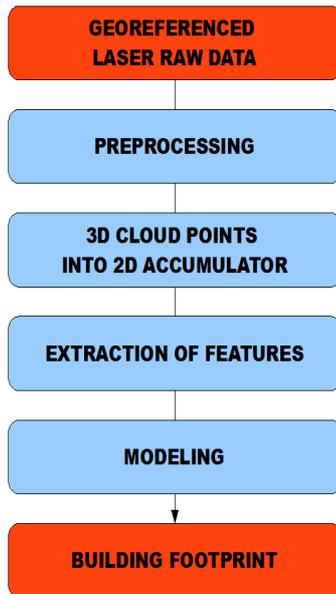
Figure 4: Data flow diagram of the building footprint extraction approach.
