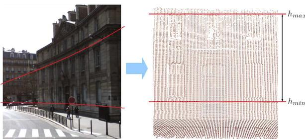
Figure 7: Acquisition of the 3D point cloud using the 2D laser sensor. The frame shows a selected band without occlusions.
