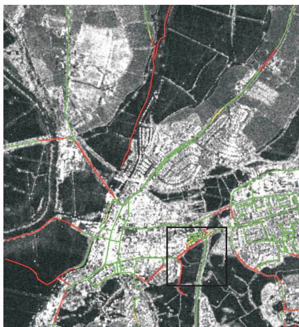
Figure 9: Automatic assessment of roads using the classification system: flooded roads (red), trafficable roads (green) and possibly flooded roads (yellow)
