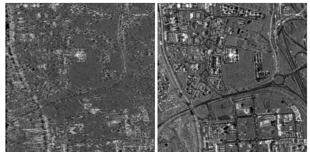
Figure 10: Simulated SAR scene obtained after 25 iterations (left) and really detected one (right)
