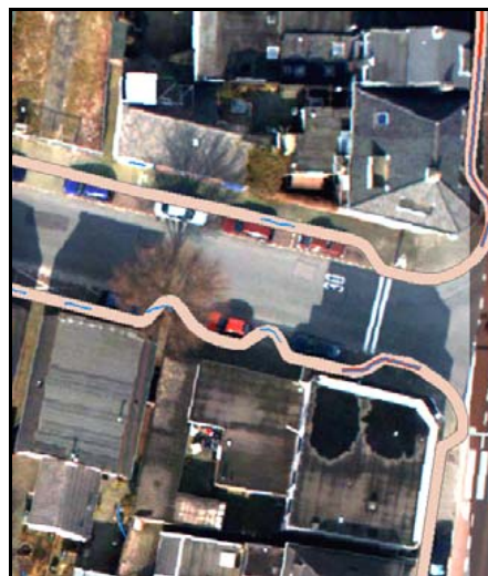
Fig. 11: Buffer around road side as manually outlined in an orthophoto (pink) with initially detected road sides (blue) and those accepted after bridging gaps and checking the segment length.
