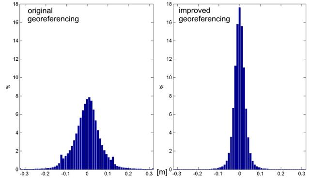
Figure 5: Histogram of the strip differences  $dZ_{pair}$  (considering the roughness mask) based on all overlapping strips (ca. 118 million values). Left: original georeferencing ( $\sigma_{MAD}=6.2\text{cm}$ ). Right: improved georeferencing after strip adjustment ( $\sigma_{MAD}=2.9\text{cm}$ ).  $\sigma_{MAD}$  is the standard deviation derived from the median of absolute differences (the so-called *MAD*) as  $\sigma_{MAD} = 1.4826 \cdot MAD$ .
