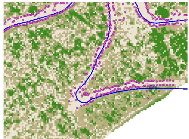
Figure 7: Result of the borderline detection. The blue line corresponds to the simplified centerline estimated from the region growing algorithm. The pink dots represent the borders correctly estimated from the cross-sections.
