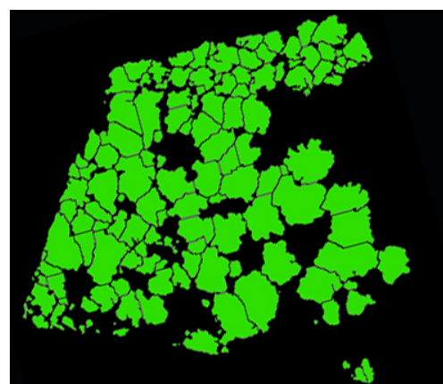
Figure 3 Segmentation result in aerial photograph based on the watershed algorithm. Each canopy is indicated as green region. Boundaries of each canopy are represented as black lines.
