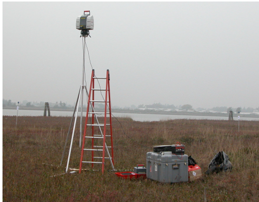
Figure 3. The tripod used to rise up the laser scanner. On left and right side two poles holding retroreflective targets are visible in the background.
