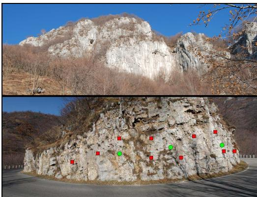
Figure 2.- Images of rock faces “A” (at top) and “B” (at bottom) where the red squares are the GCPs and the green circles are the independent check points.
