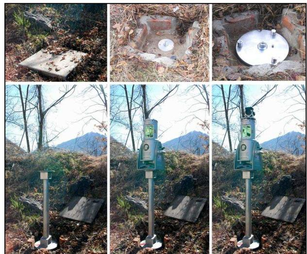
Figure 3.- Main steps of the installation of the TLS stand-point.
