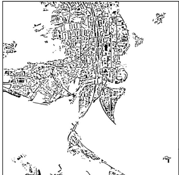
Figure 4. Result of a modified Laplace filter operation conducted with IMALYS. In combination with a dataset as shown in Figure 3, this kind of information can for example be used to discriminate different residential sealing classes.
