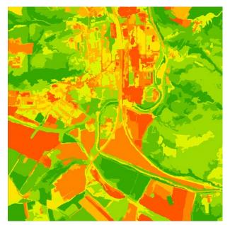
Figure 3. A sample result of the IMALYS feature retrieval. Depicted is the NDVI of each cell. The more greenish colors represent cells with higher vegetation activity.
