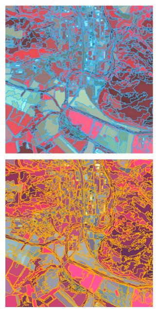
Figure 2. Sample results for the segmentation algorithms implemented by IMALYS. The upper image displays a result of the region-growing approach; the lower image shows a segmentation conducted by using the watershed algorithm.
