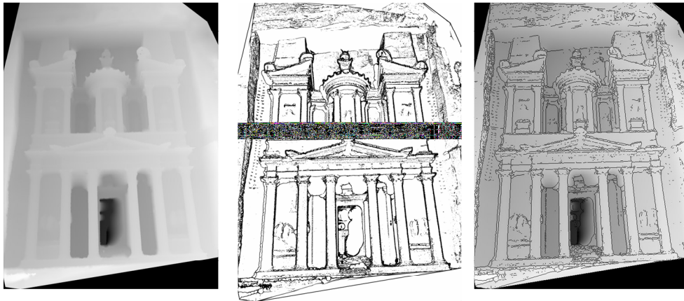
Figure 7. a) Range image collected from Petra treasury (Al-Khasneh). b) Segmentation results using mask size 11. c) Edge map projected in the range image after skeletonized.
