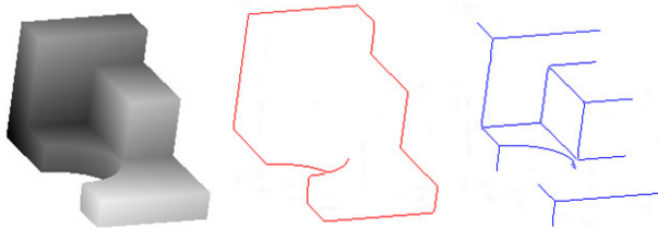
Figure 4. Curve block segmentation using different thresholds to detect step edges (red) and crease edges (blue).
