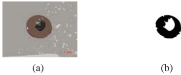
Figure 5: Segmentation of Fig 1(a): (a) A single segmentation obtained using the using mean shift algorithm with parameters h_s = 7 and h_r = 11 , and (b) mask created from a single segment in (a).
