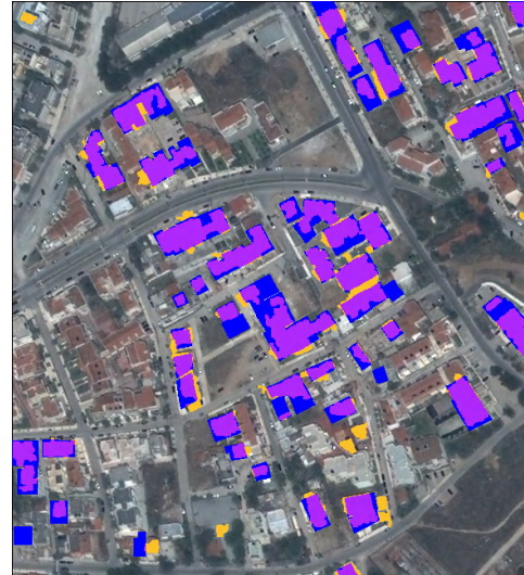
Figure 4. The purple pixels referred to the classified buildings of the original image data, the yellow pixels indicated the false alarms (False Positive: 5369pixels) and the blue pixels indicated the undetected pixels (False Negative: 16075pixels).
