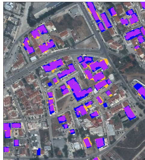
Figure 5. The purple pixels referred to the classified buildings of the filtered image data, the yellow pixels indicated the false alarms (FalsePositive: 4744pixels) and the blue pixels indicated the undetected pixels (FalseNegative: 13678pixels).
