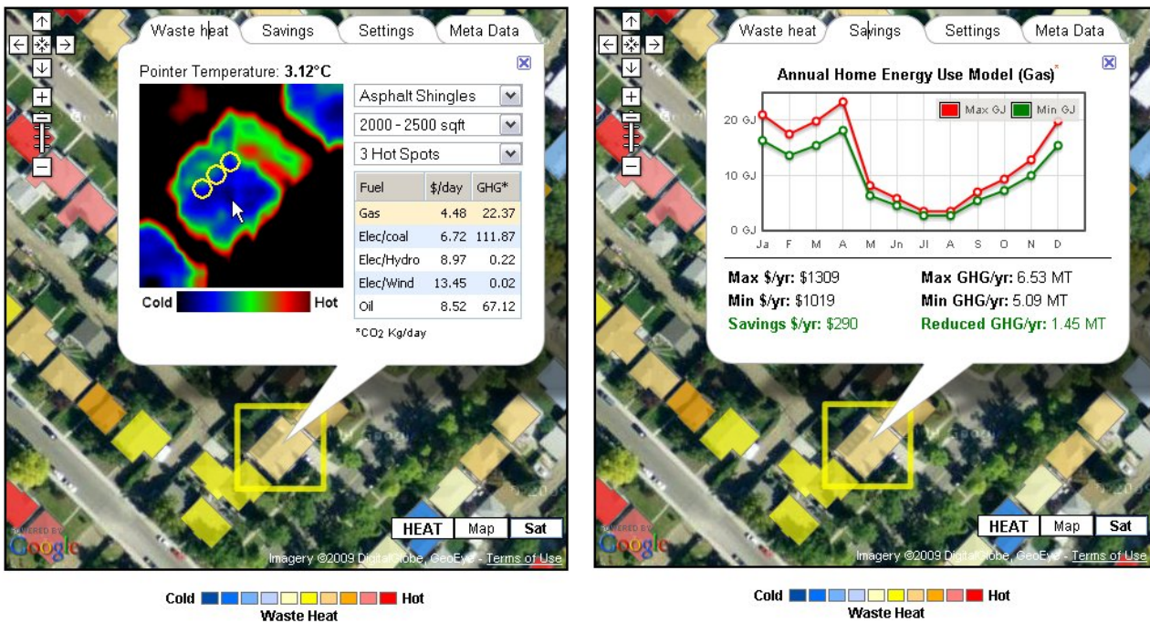
Figure 1. Yellow circles ( Left ) automatically define the 3 hottest locations on a home – which in this case fall above 4 sky-lights. The colored polygons (that overlay the image) are from a residential database, and are color based on the average roof-top temperature. This allows for neighborhoods to be evaluated at coarser scales. The mouse-over pointer value (3.12 °C) is dynamic, and the energy use-model estimates GHG and cost/day to heat this home to the maximum defined temp using different fuel types. When Natural Gas (in tan highlight) is double clicked, a model is generated ( Right – Savings tab ) for this home/year with total costs as well as GHG and savings based on reducing waste heat to the min roof temperature defined by the thermal sensor (prices shown are examples only).
