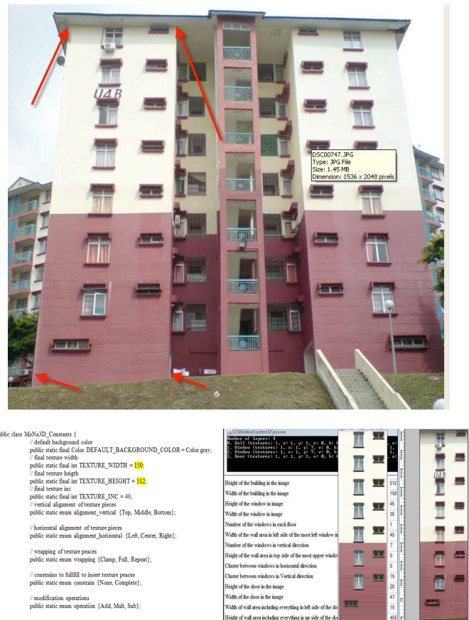
Figure 2. Four points must be selected in a plane with known coordinates where each point provides 2 independent equations (1.1 and 2.1)
