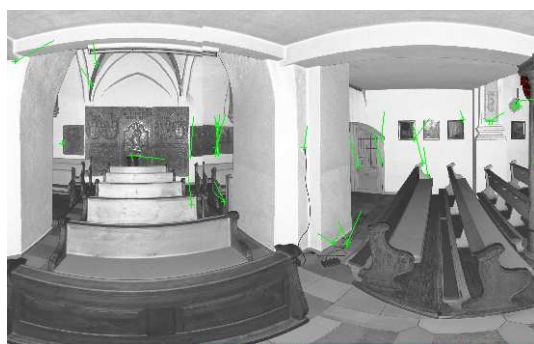
Figure 8: External camera calibration: (a) Statistical measures after outlier detection with ransac (b) Scaled error vectors of the feature extraction and matching approach
