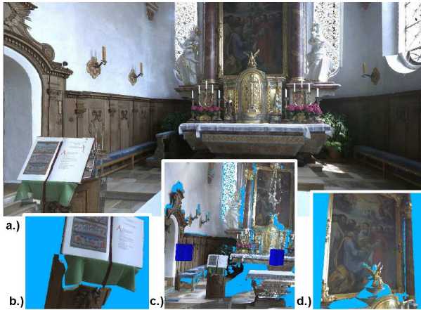
Figure 10: Kirche Seefeld: Colored 3D point cloud (ii)
