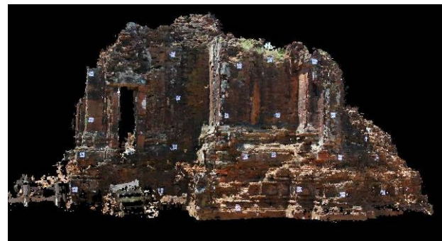
Figure 14. The point cloud extracted with PhotoModeler Scanner by using orientation parameters computed with the proposed S&M algorithm.
