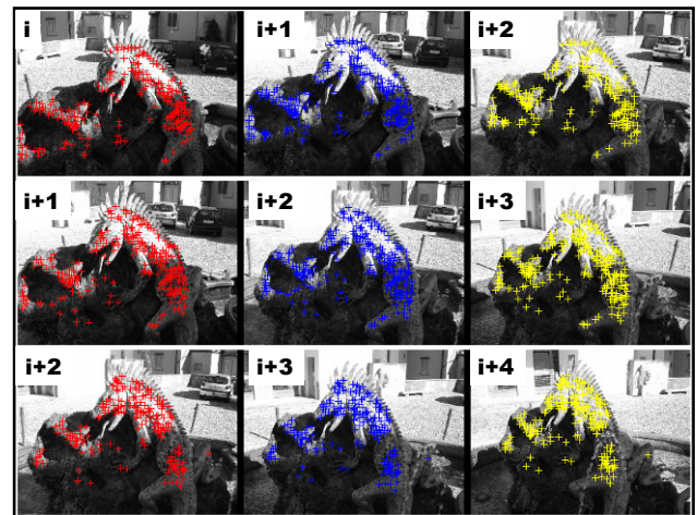
Figure 3. Three consecutive triplets of an image sequence and the extracted tie points by F.-B. Matching.
