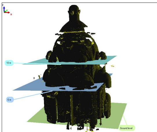
Fig 5 - Scheme of the scaffoldings and the survey levels
