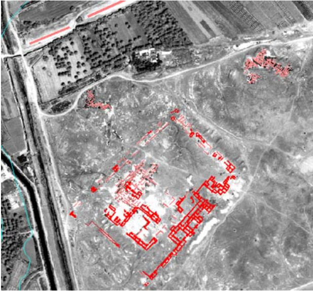
Figure 6. Sippar: a detail of an Ikonos orthoimage (23-05-2002) with vectorization of ancient traces and remains.
