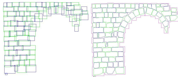
Figure 7. Blocs bounding boxes scaled at 1.25 (left) and the computed perimeter displayed in magenta (right) superposed with the original blocs.
