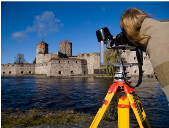
Figure 2. Panoramic head mounted on a standard geodetic tripod
