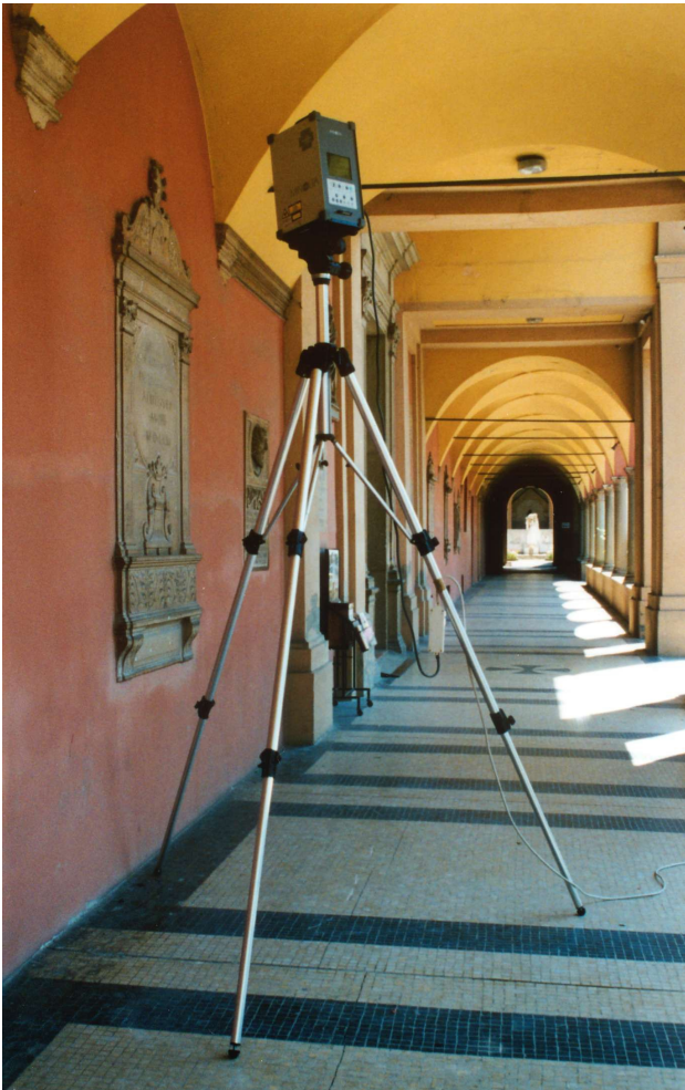
Figure 8. The experimental setup for 3D laser scanning of the gravestone in the front of Certosa church.
