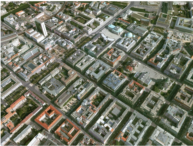
Figure 1: Rendering of the automatically reconstructed city model of downtown Berlin on top of a corresponding DSM.
